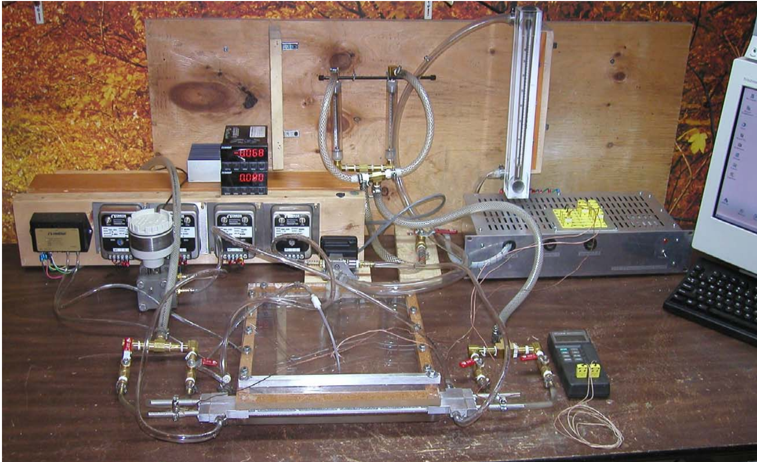
COUNTER FLOW HX UNIT UNDER TEST
