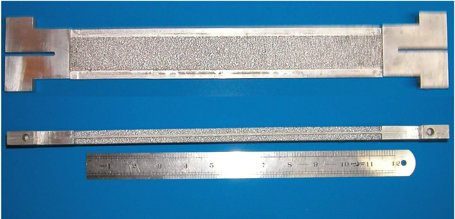
RMF Based 1KW Air to Liquid HX, 0.3 lb, 5.3 in 3 (0.003 ft 3 )
